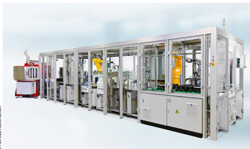
Figure 3 > Ten meters long and four meters wide, the system houses 21 active modules.
