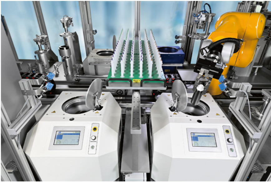
Figure 4 > Vacuum speed mixers enable precise mixing and complete deaeration of high-viscosity formulations, even in small quantities.
